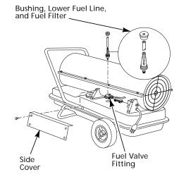
Figure 11 - Fuel Filter Removal
